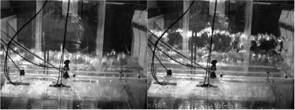
FIGURE 6. Growth of three-dimensional effects during the water rising up the vertical wall. View towards the incident waves. Time increases from left to right and the time interval is \Delta t = 0.08 s.
